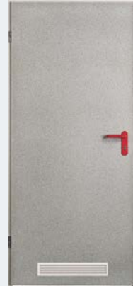
Ventilation grille A 458 x 92 mm grille is positioned at the bottom. On request, the grille is also available at the top of the door. (Only for ZKS/ZKD doors)
