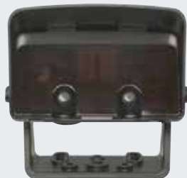
Radar movement detector MWD-C Fast and targeted automatic door opening, directional recognition, max. fitting height 7 m, fitting in cold store possible up to max. -22° C, housing protection category IP 65
